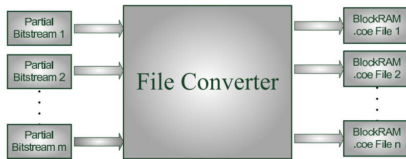
Figure 4.5. File conversion from partial bitstream file to BlockRAM coefficient file.
