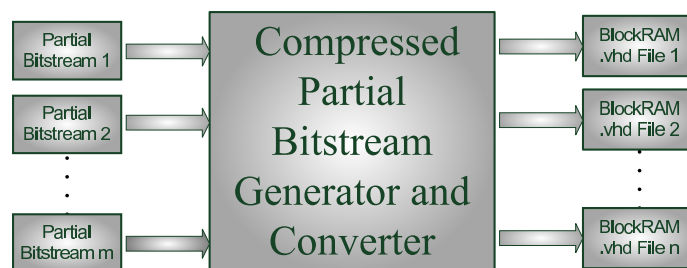
Figure 5.4. File conversion from partial bitstream file to BlockRAM coefficient file.
